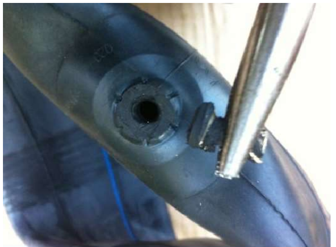
8. Notice how smoothly the cut is around the stem - this will help keep it from tearing when the new metal stem is installed and later when the tube is inflated
