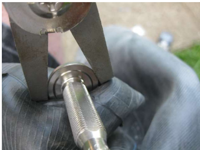
15. These pliers open it up just enough to get the stem started in the hole
