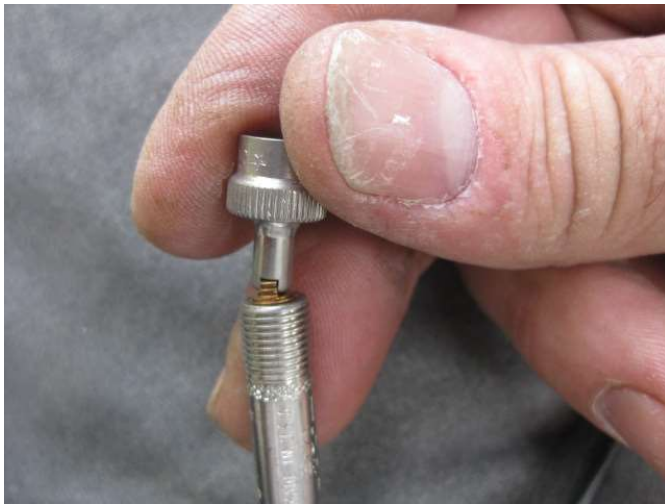
19. Put in a new Schrader valve (particularly if using old stems), and tighten the valve with the cap
