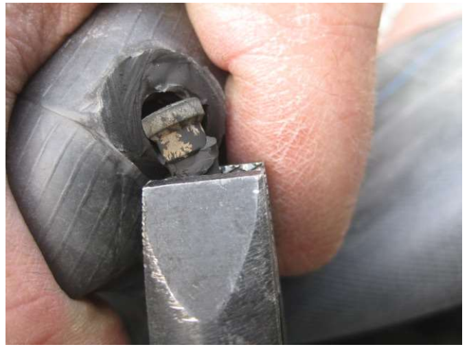
6. Twist the brass tube out. Cut around the edge if needed (see next step below), but the goal is to leave the inside of the hole as round and smooth as possible
