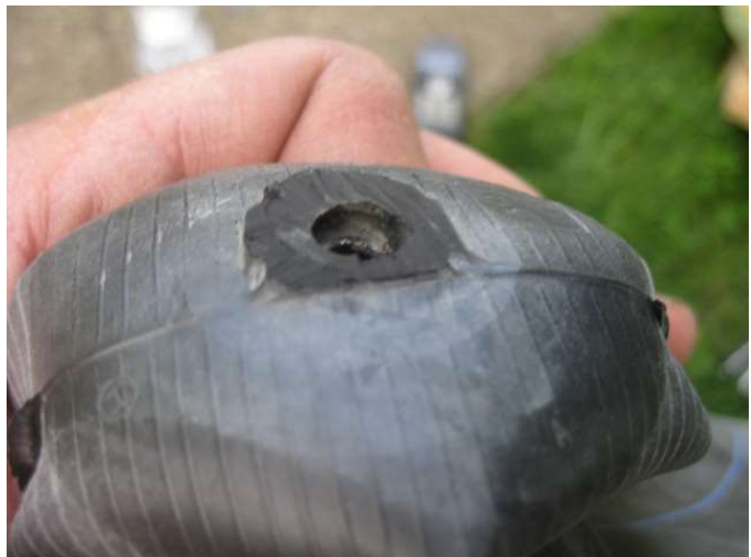
10. Try to end up with something reasonably flat and close to the surface of the tube
