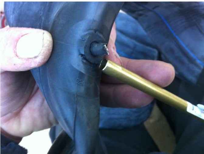
7. If the brass stem is not easy to remove, it will be necessary to cut it out so that the tube doesn't tear and ruin. With a razor blade it is hard to keep it round and this leaves places where it can tear. However, you can use some 5/16" brass tubing to cut around the stem
