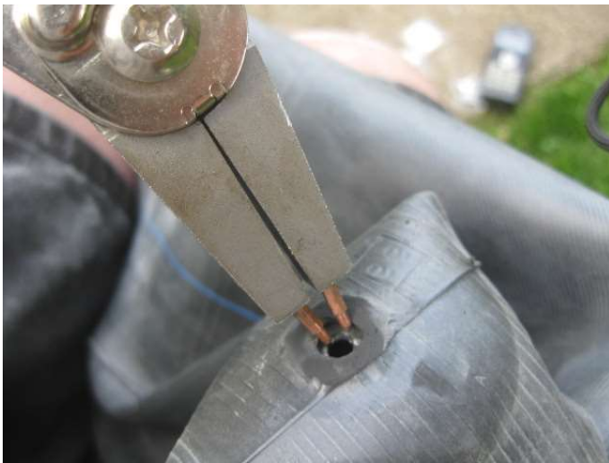
13. Use snap ring pliers or just needle nose pliers to open up the hole
