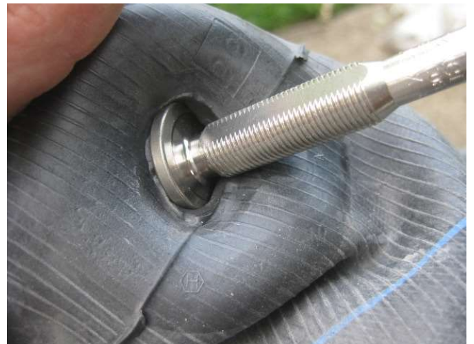
16. Once the stem is in the hole the pliers can be removed to finish inserting the stem
