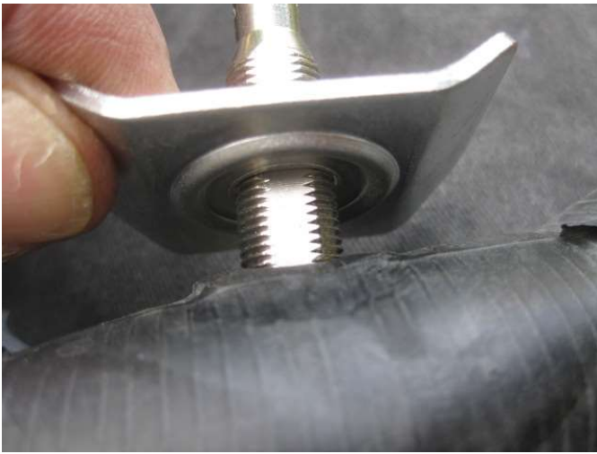
17. Put on the bridge washer. The ridges in the stem base and the bridge washer are enough to seal the air from leaking. You might use bead sealer if you have some handy
