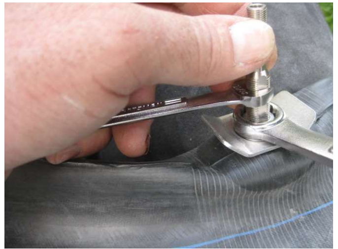
18. Place and tighten down the nut. I've heard some people express concern about making it too tight and squeezing out the rubber from between the washer and the base but I don't see that happening when I get it good and tight by hand. Make sure the stem and washer stay in line with the tube and don't turn as you tighten
