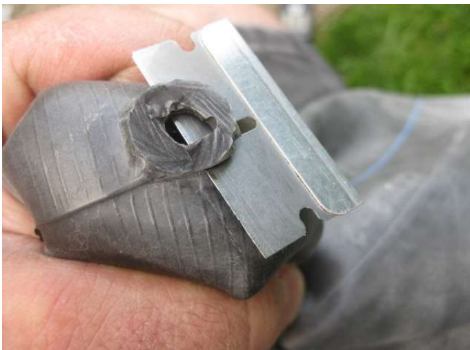
9. Trim close to the base. These multiple extra cutting steps are not necessary if the brass tube was easy to remove and don't want to tear up the tube
