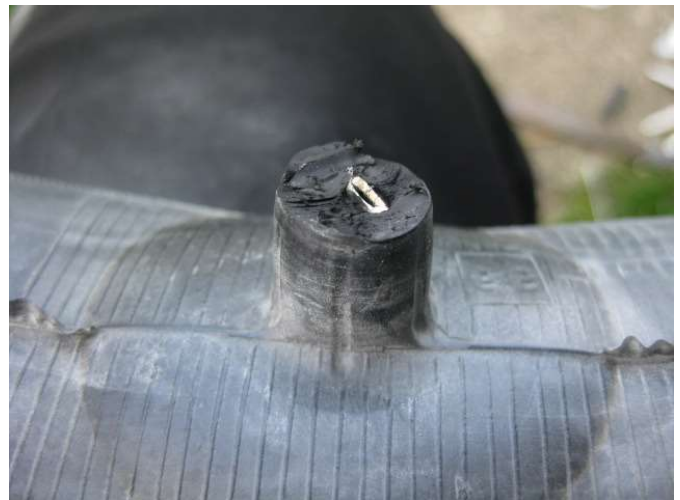
2. This leaves a stub with the (now crushed) brass tube in the center
