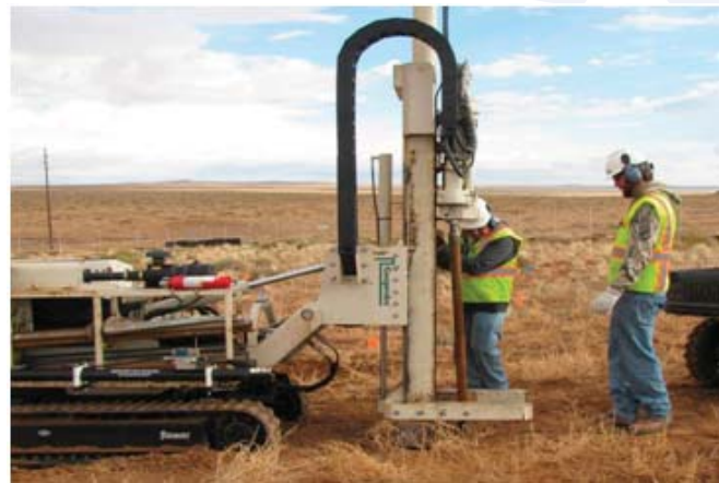
A test hole being punched using the Geoprobe.
