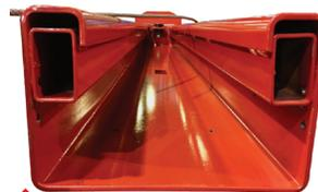
2.5" x 1.5" (63mm x 38mm) column reinforcement tube
