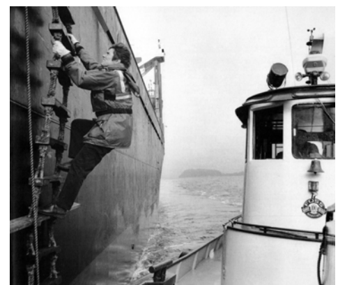
Retired Columbia River Bar pilot and JDC member Captain Deb Dempsey climbs the pilot ladder after a transfer from the pilot boat. Photo by Jill Johnson.
