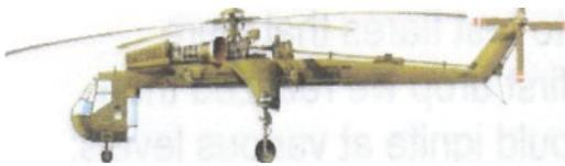
During our mission the remains of a CH-54 accident (6 January 1966) was being recovered. The aircraft accident happened because the crew had left about 100 feet of cargo line trailing behind the aircraft. The line tangled in the tail rotor causing one of the main rotor blades to separate from the aircraft. This was the first accident of a CH-54 aircraft.
