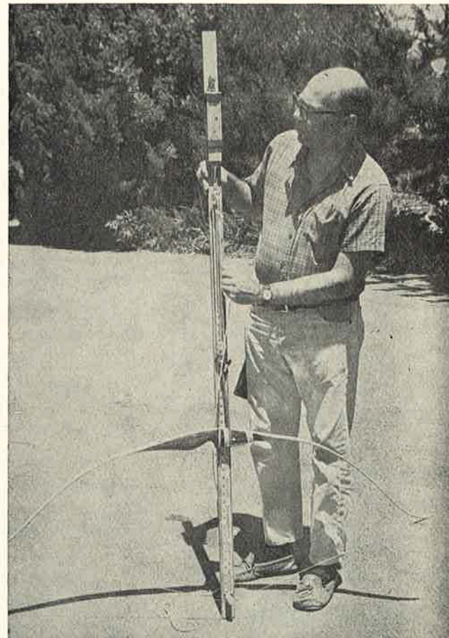
FIGURE II: Bow being drawn along yardstick while force in pounds is recorded from scale reading.
