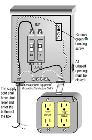
The disconnect may be permanently installed within a concession stand or mounted to a portable backboard.
