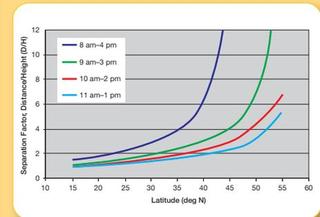
Figure 22. Multiple rows of rack mounted PV arrays must be separated to prevent shading.
