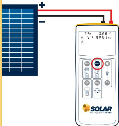
Polarity should be verified on the following dc components and circuits PV system:
