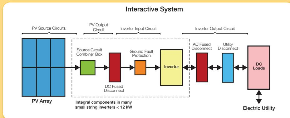
inverters can provide stand-alone power for critical loads independent from the grid during outages. See Figure 16.
