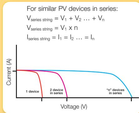
Connecting PV modules in series with dissimilar current ratings results in loss of power, similar in effect to partially shading an array, or having parts of a series source circuit located on surfaces facing different directions and receiving different levels of solar irradiance. The resultant
