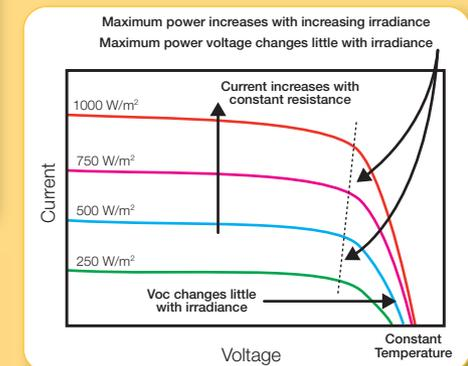
Therefore, doubling the solar irradiance on the surface of the array doubles the current and maximum power output (assuming constant temperature). Changing irradiance has a smaller effect on voltage, mainly at lower irradiance levels. Because voltage varies little with changing irradiance levels over 200 W/m<sup>2</sup>, PV devices are well-suited for battery charging applications. See Figure 5.
