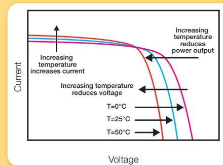
Since PV modules produce their highest voltage at the lowest temperatures, this voltage determines the minimum voltage ratings required for the modules and associated dc circuit components [NEC 690.7]. For crystalline silicon PV modules, the maximum voltage for PV arrays
