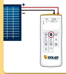
Polarity should be verified on the following dc components and circuits PV system:
