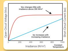
The short-circuit current (Isc), maximum power current (Imp), and maximum power (Pmp) at one condition of solar irradiance may be translated to estimate the value of these parameters at another irradiance level:
