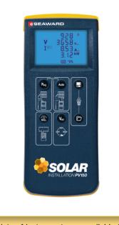
A variety of instruments are available for the PV installer, but it is important to make sure the correct instrument is selected and avoid products which only provide one or two tests, reducing the number of instruments needed as well as calibration requirements. The Seaward Solar PV150 is a hand held meter that performs a variety of tests in a safe and simple fashion.
