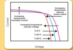
Since PV modules produce their highest voltage at the lowest temperatures, this voltage determines the minimum voltage ratings required for the modules and associated dc circuit components [NEC 690.7]. For crystalline silicon PV modules, the maximum voltage for PV arrays
