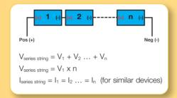
Figure 9. Connecting similar PV devices in series increases voltage while current stavs the same.
