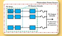
A string is a series connection of PV devices. PV cells or modules are configured electrically in series by connecting the negative terminal of one device to the positive terminal of the next device, and so on. For the series connection of similar PV modules, the voltages add and the resulting string voltage is the sum of the individual module voltages. The resulting string current output remains the same as the current output of an individual module. See Figure 8 & Figure 9.
