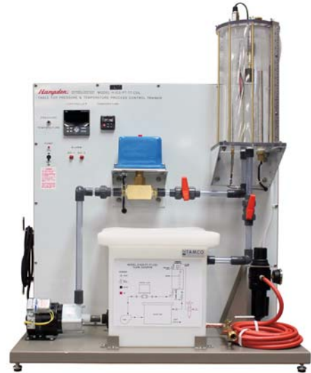
MODEL H-ICS-PTT-TT-CDL Pressure and Temperature Process Control Trainer
