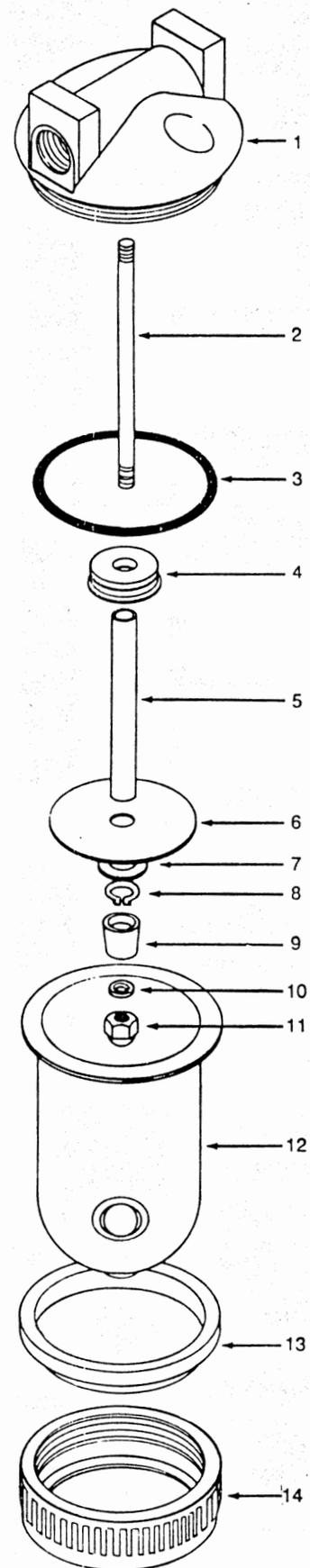
**NOTE:** If excessive pressure drop occurs, replace exhaust element, (1170-12 or 1170-15)
