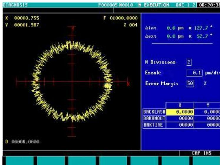
If the machine parameters are protected, it will request the access password because the bottom right of the screen shows some of them. When not knowing the password, those values cannot be changed, but it will be possible to access the screen and the circle geometry test.
