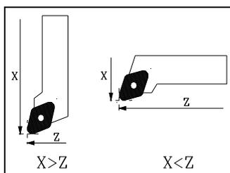
If the "X" length assigned to a tool is greater than the "Z" length value, the CNC will show a tool with a vertical handle and when "X" is shorter than "Z", with a horizontal handle.
