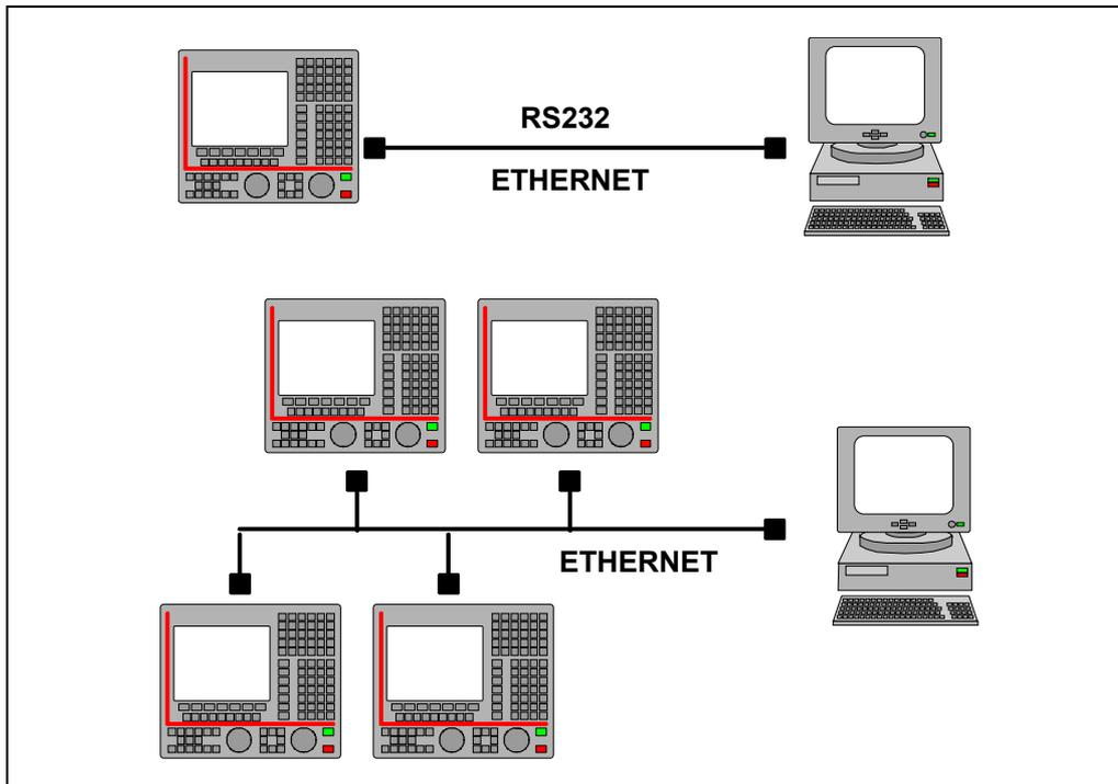
For the RS232 connection, the remote PC must have the WinDNC software (version V2.00 or later) installed in it. For the Ethernet connection, the remote PC must have the WinDNC software (version V4.00 or later) installed in it.
