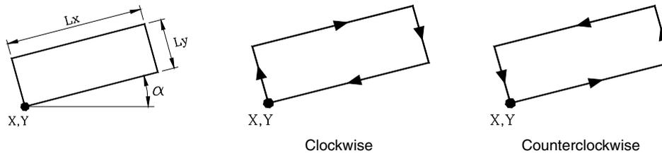
A straight angular profile is defined with a single command, but the CNC internally breaks into 4 straight segments.
