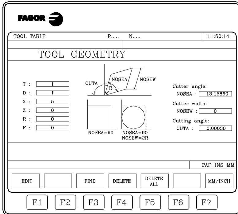
The data corresponding to each tool is contained in the following fields:
