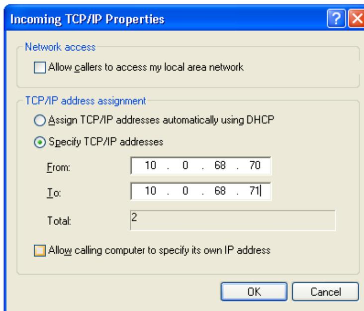
Indicate the TCP/IP addresses. Enter in the "From" field an address that belongs to the local network where the PC is and in the "For" field the next one.
