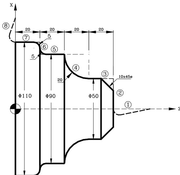
**Profile definition without rounding, chamfers or tangential entries and exits.**
