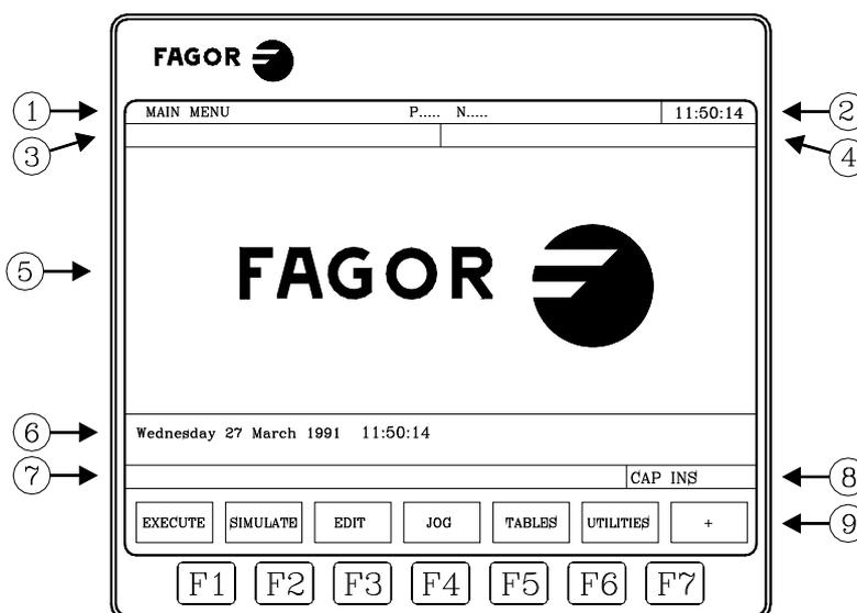
1. This window indicates the selected operating mode, as well as the program number and the number of the active block. The program status is also indicated (in execution or interrupted) and if the DNC is active.
