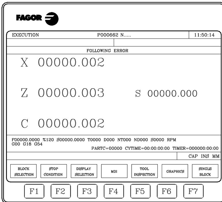
The display format is determined by the axis machine parameter "DFORMAT".
