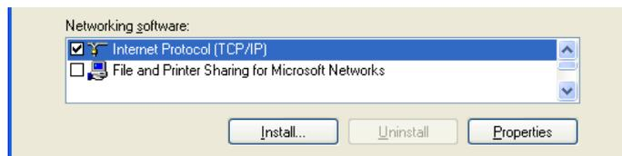
Select the TCP/IP protocol from the list of components and press the properties button.
