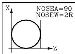
When the cutter is round, the cutter angle will be 90 (NOSEA=90) and the parameter corresponding to the cutter width must be assigned its diameter value (NOSEW = 2R).
