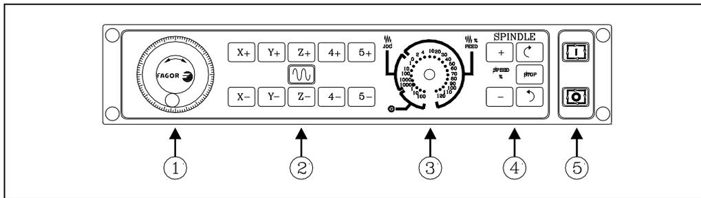
1. Position of the emergency button or electronic handwheel.
