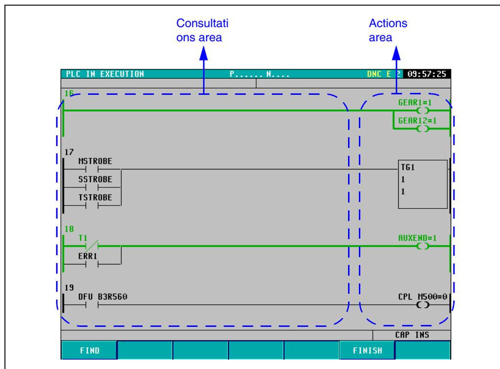
As shown in the figure, the instructions of the PLC program in ladder language is made up of elements connected to each other by segments. It also shows the logic way for the flow highlighted with a thicker green line and shows the values of registers, timers, counters, etc.
