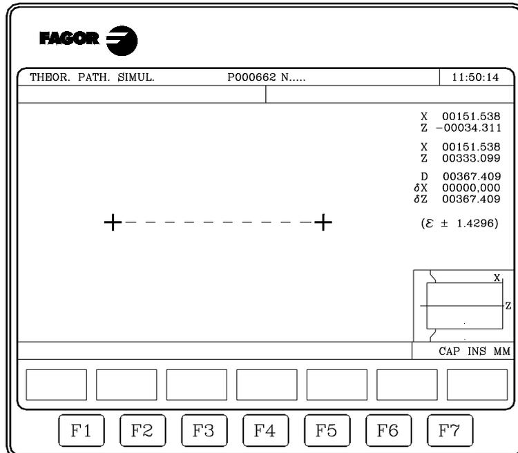
The center of the CRT shows a dotted line with two cursors, the section to be measured. Also, the right-hand side of the screen shows:
