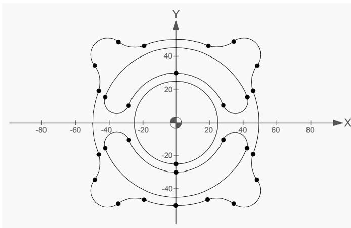
The profile graphics takes into account the value of general machine parameter GRAPHICS (P16) to determine the direction and position of the axes.
