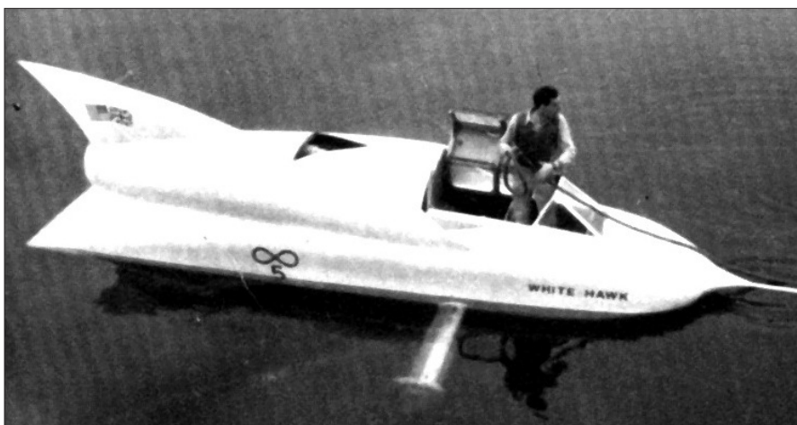
The White Hawk jet hydrofoil built by Frank and Stella Hanning-Lee
