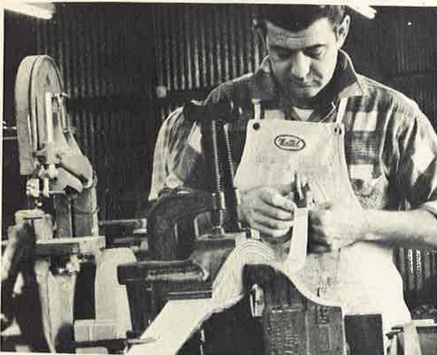
5. Craftsman Rathbun uses epoxy glues to add tips to the blank form after removal from the drying form. These hardwood riser laminates and bow tips add beauty and strength to finished bow. Here, it is in early manufacture.
