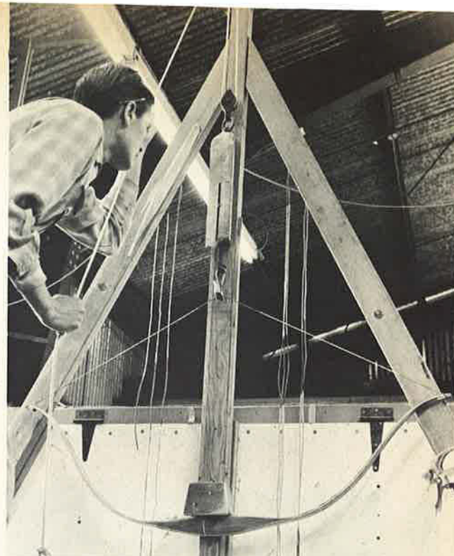
14. Again, since conventional machinery would not afford desired results, the FASCO bowyers designed this 118-inch vertical sander. Sight window is rough sanded on this machine until the final shape of bow begins to appear.
