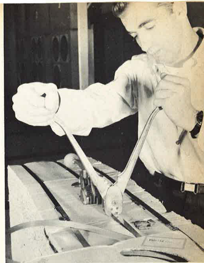
A fastener is applied to the bands to hold together.
