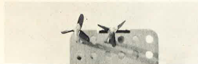
The arrow visible on the left boasts a helical fletch, while the one on the right was fletched with a straight clamp on an angle. Note larger frontal area on helical.
