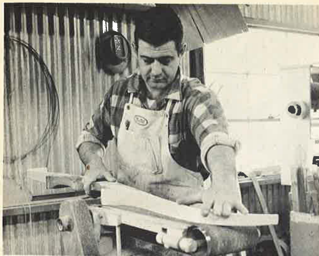
10. Above: Horizontal sander removes some of the rough edges and shape of bow becomes more evident. (Right) Bruce McCall uses pulley system with scale to check the weight of a bow. Here, weight and alignment are critical.
