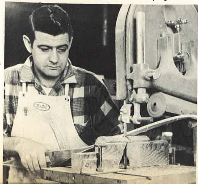
8. Rathbun uses bandsaw to cut scribed blank along the pattern. Bandsaws have rests on them for the blank to run through as bowyer cuts the shape of the limbs, forms window, makes fine cuts to add to first shaping of bow.
