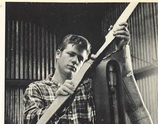
12. Jim Keller uses vertical sander to rough shape a bow after McCall has finished first alignment. This brings out grain, beauty of the wood, which has been underdeveloped during many stages the bow has previously undergone.
