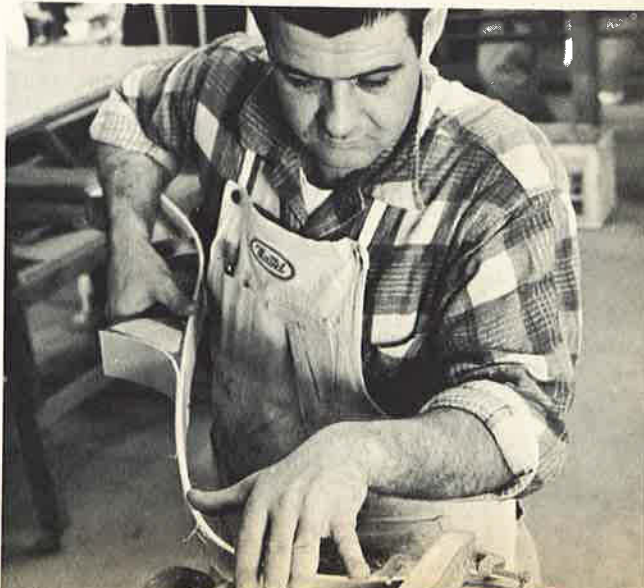
9. The use of a special machine gives the bow blank its first cut in the process of making the rough grooves for the string. This wheel is guided by a jig that is so designed that it consistently gives same results to bows.
