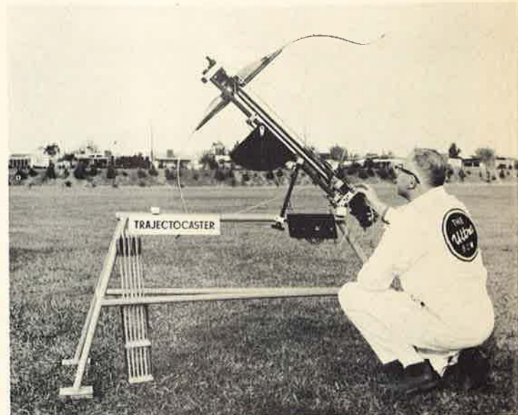
BOW & ARROW's Tom Jennings is ready to touch one off. So as to create as little movement as possible, the arrow is released by actuating a special camera cable release.
