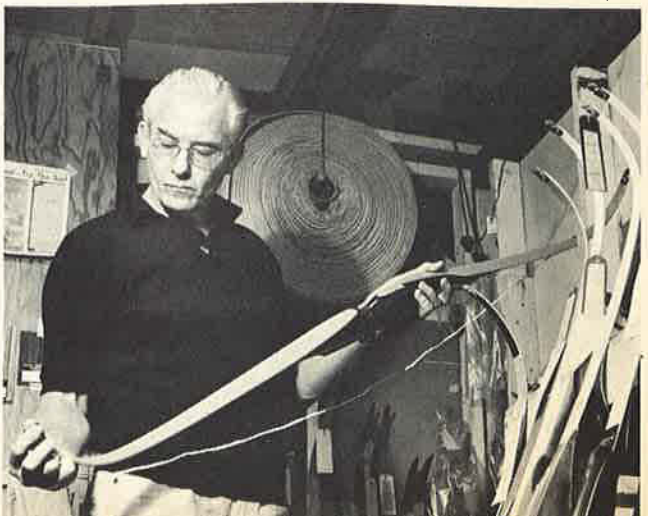
21. Carl McCall checks the finished product prior to its being wrapped for shipment. Taken into consideration are alignment, finish and general quality. Each bow also is fitted with dacron string before shipment to a buyer.
