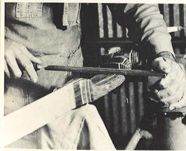
15. A wood file is used to file the fine surface on the bow's sight window. This assures a smooth, flat surface from which the future owner can shoot. Despite amount of specialized machinery, much hand work still is required.
