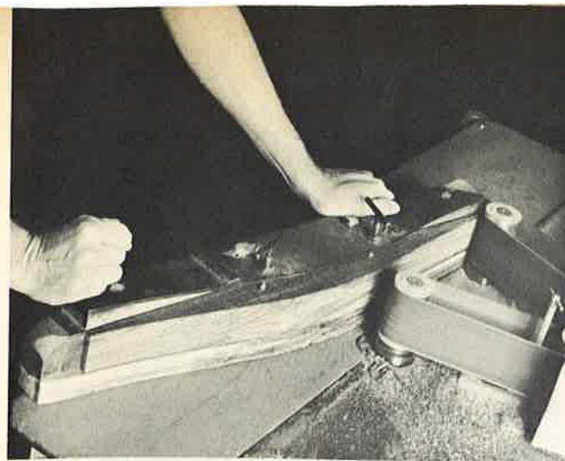
2. Anderson uses specially built sander with template to give riser wood its initial shaping. Template insures uniformity in each riser. The sander was designed to speed the work without sacrificing any quality in workmanship.
