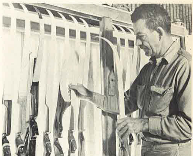
19. Bows are removed by Mart Mathew after spray with epoxy and placed in drying cabinet. This finish not only adds to the bow's beauty, but has a practical use in that it protects the woods and laminates for countless years.
