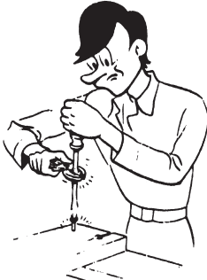
Fig. 6-13. Don't use pliers on the shank of a screwdriver to remove a stubborn screw.
