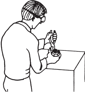
HEAVY DIAGONALS ARE FINE FOR CUTTING THE SPREAD ENDS OF COTTER PINS.
