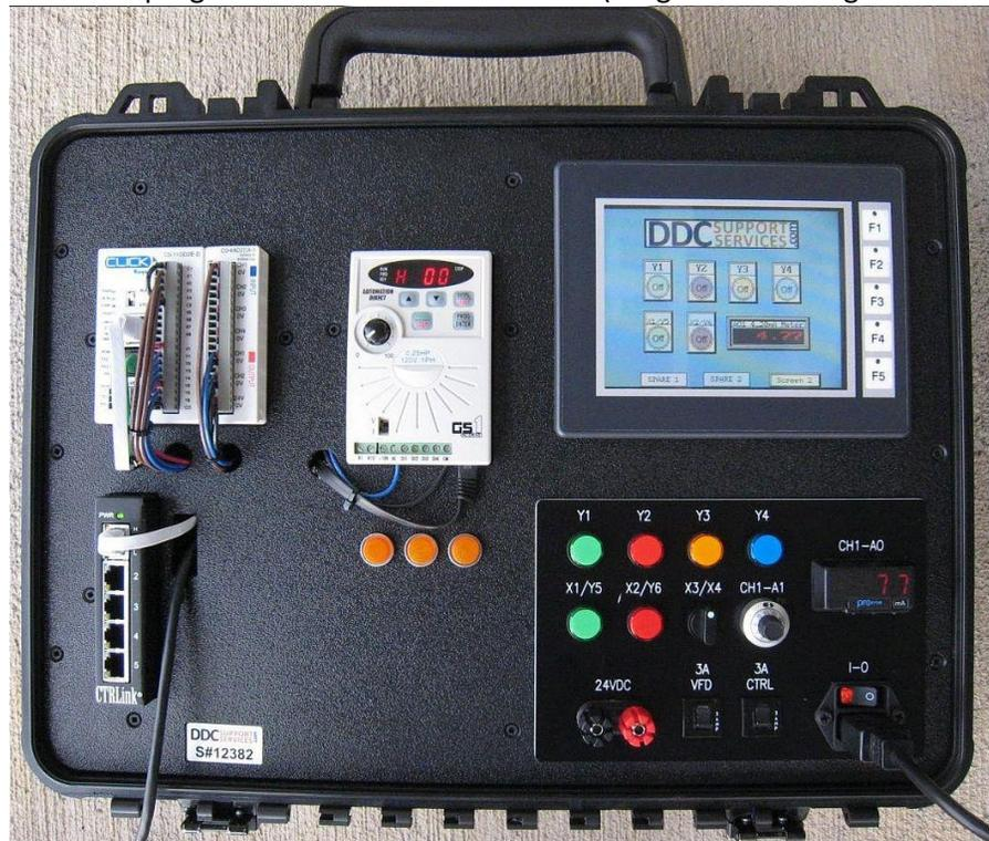
has RS-232 and RS-485 ports for Modbus RTU communication. It also has integral discrete Input/Output and an analog expansion module for 4-20mA device interface. The color touchpad display can be
