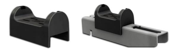
**Polymer Cable Saddles** are made from injection molded glass-filled Polymer resin to create a strong, non-conductive cable saddle for use with underground cable support arms in vaults and manholes. The fiber-reinforced polymer saddles are non-corrosive for long-term durability. Emits no harmful smoke. Secures the cable tightly to the saddle.
