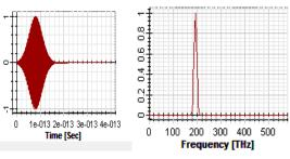
Fig. 9: Gaussian Input Source
