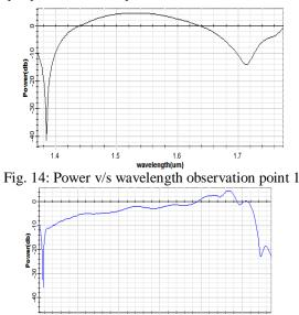
$^{14}$   $^{15}$   $^{16}$   $^{17}$   $^{18}$ Fig. 15: Power v/s wavelength observation point 2 The output is possessing less ripples in comparision to concave taper and observed a bend at 1.55µm. The output is many fold smoother than the previous output. *E. Exponential taper*
