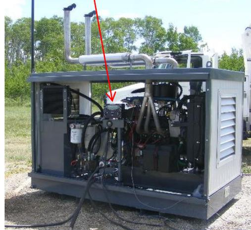
Custom Designed Non-Contact Sensor Bar
