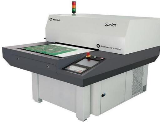
Powered by **Orbotech DotStream Pro Technology™**, Sprint systems deliver cost-effective, top quality industrial inkjet printing for a consistently accurate production of even the most advanced legend designs to meet any manufacturing volume need.
