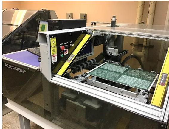
Our Accu-Score AS-150-MAX V-Scoring Machine is designed to score continuous and segmented ("jump") v-grooves on one or both sides of any type of PC board substrate.
