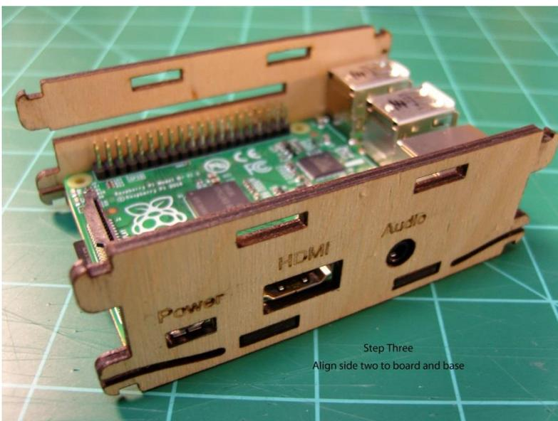
**Three** – Add the second side, line up slots with inputs/outputs
