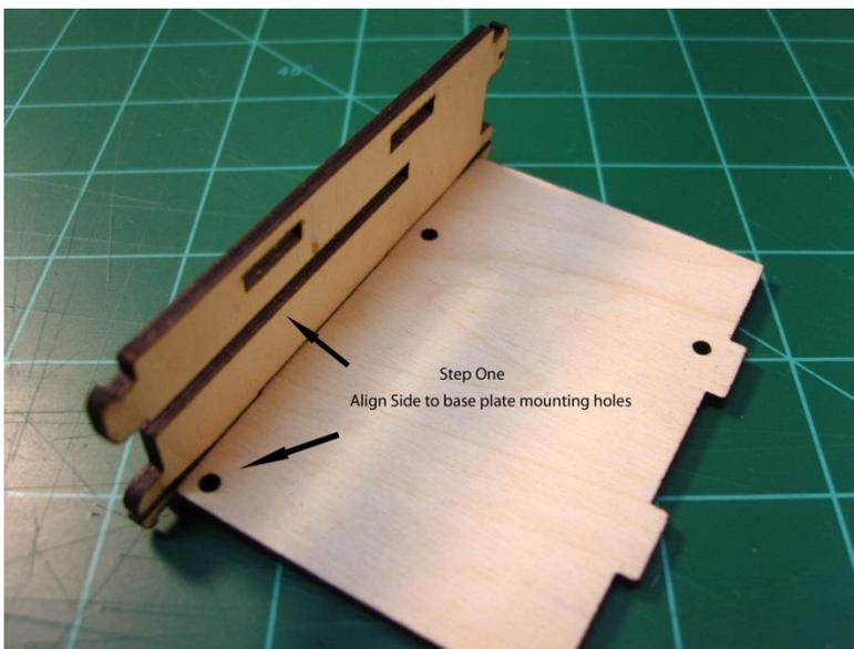
**One** – Line up side with base, use slot and holes to assist
