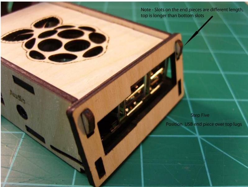
**Five** – Attach USB/Ethernet end plate, start by placing slots over top lugs - note slots are different length at top compared to bottom
