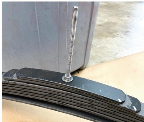
All-thread rod used to compress the leaves to complete the spring stack
