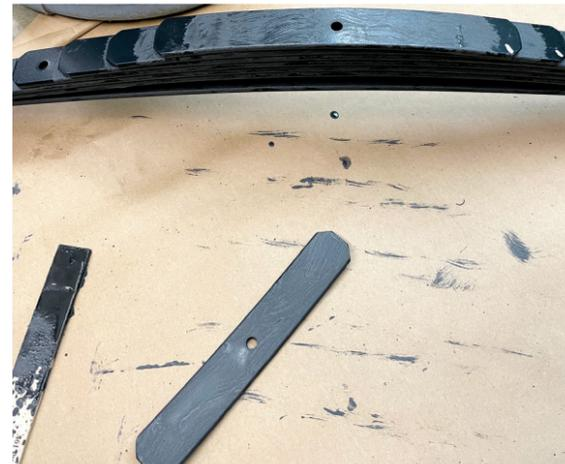
Each leaf marked to identify its mate in the stack, and the contact surfaces above and below each leaf coated with dry lube.
