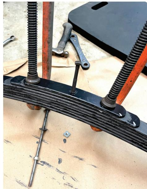
Now the new front spring is completed with dry film lubricant between the leaves and ready to receive a nice finish coat of shiny black enamel and install on the T. The dry lube should last and last.
