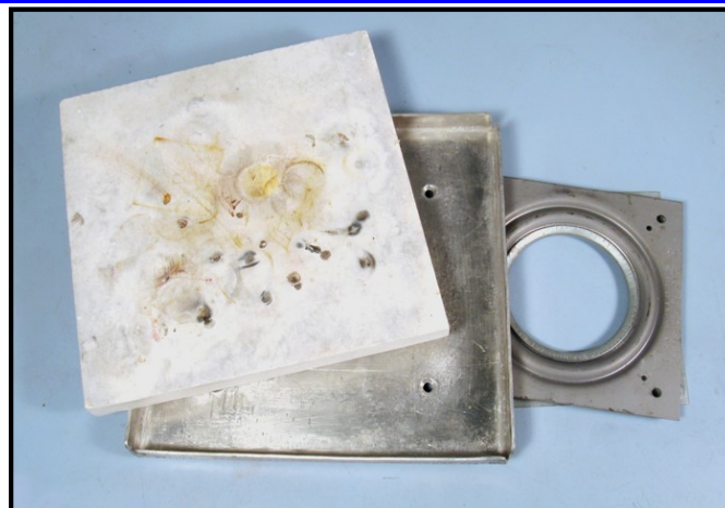
The three basic parts to the rotating soldering pad
