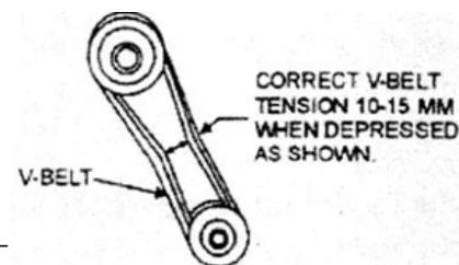
Figure 2. V-Belt Tension
