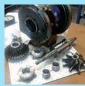
Customer-supplied Turboexpander-Compressor for evaluation and repair.
