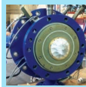
Turboexpander-Compressor mechanical center section (MCS) redesigned for increased flow and efficiency.
