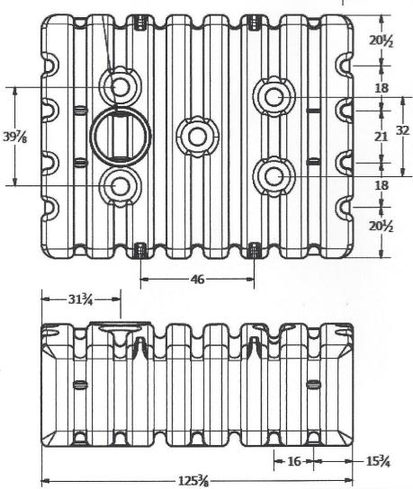
D Systems uses the largest capacity below ground storage tanks made today. Used to store water - both potable and non-potable for a number of applications. The end ribs will accept fittings up to 4" in size. Integral columns in the tank give it excellent structural strength.
