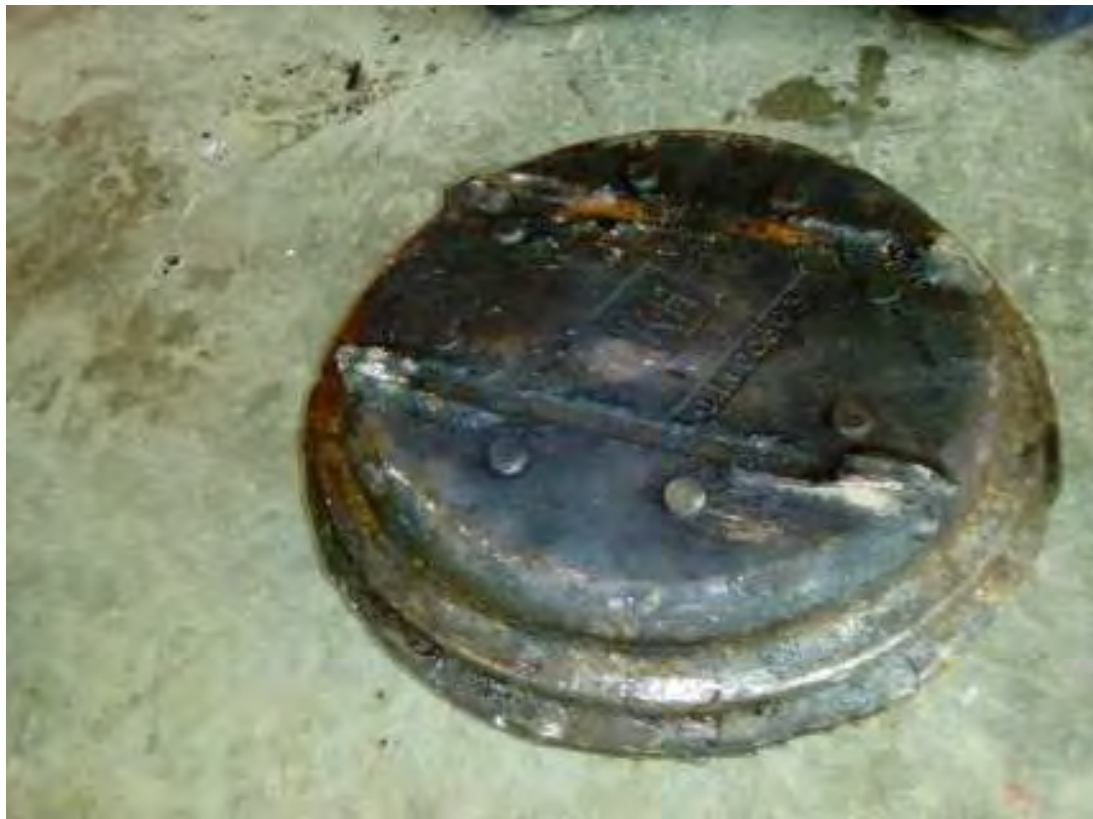
Photo 3 King pin and housing at initial inspection
