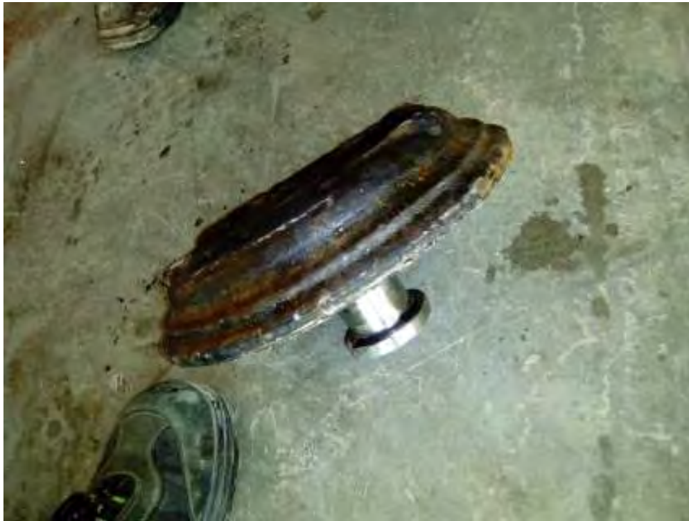
Photo 4 King pin and housing at initial inspection
