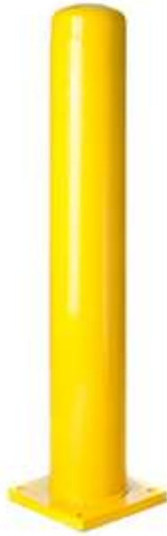
6" O.D. x 42" or 48" on a 10" x 12" base plate 1/2" thick with four 3/4" corner holes
