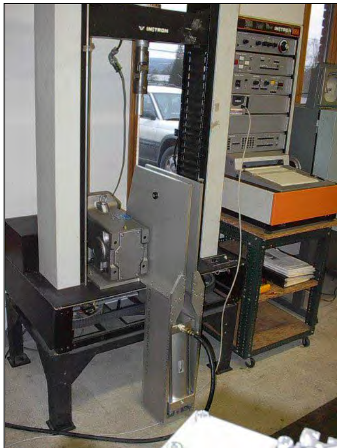
Figure 2: Rope tester mounted on Instron.
