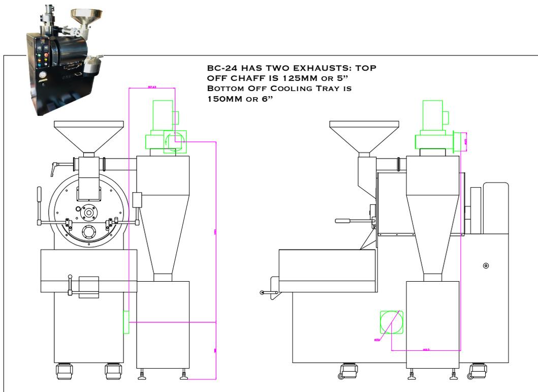
**A STANDARD SETUP OF THIS TYPE DOES NOT REQUIRE ANY MORE EXHAUST
