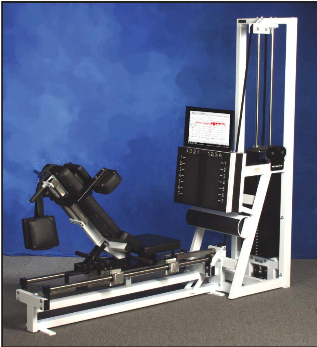
A RenEx Leg Press Machine incorporating four load cells, junction box, force meter, computer, monitor and analog interpolation software.
