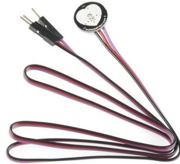
Fig.3: Pulse Sensor Cables
