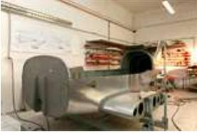
Wings attach outboard of the step area with large bolts.
