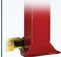
gusseted base plate requires a minimum of 4" reinforced concrete at 3500 psi
