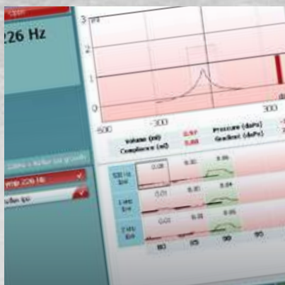
Tympanogram and reflex test results displayed simultaneously
