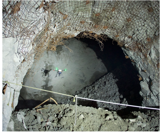
Autonomous flight into a stope
