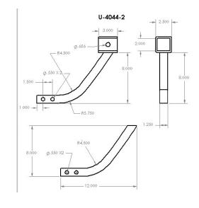
ATV/UTV Hitch 1 1/4" Hitch Riser/Extender that features a tow plate with 2 holes; one for a ball hitch and the other hole can accommodate a yard cart or other trailer with a y hitch.
