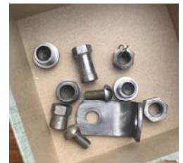
Parts after cleaning, ready for parkerizing
