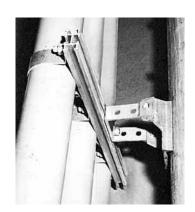
A multi-purpose bracket for mounting 1" thru 6" conduit in a variety of ways. This bracket will mount up to six 6" conduit with infinite adjustability. 4 way T-Slot extrusion eliminates field drilling. Mounts to the pole on 35/8" hole centers with 5/8" thru bolt and 1/2" lag screws (not supplied)
