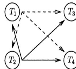
Fig. 1. Illustration of radio signal paths in an example wireless network with terminals  $T_1$  and  $T_2$  transmitting information to terminals  $T_3$  and  $T_4$ , respectively.
