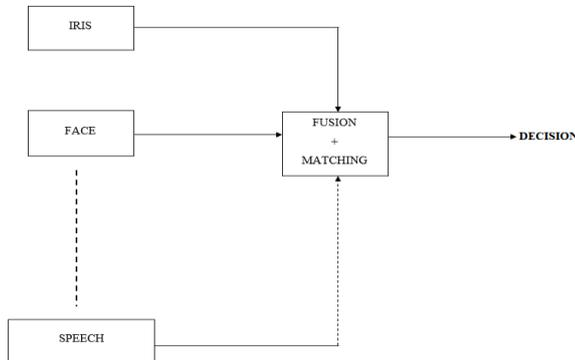
Fig.3: Parallel Architecture
