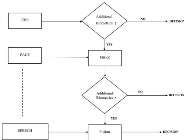
Fig.2: Serial Architecture
