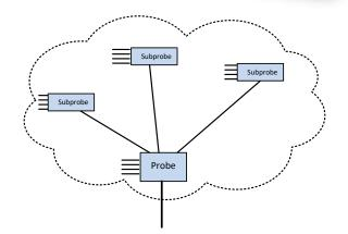
To a user of the probe, the subprobes are generally invisible; the probe determines what it needs to access for the intercepts that are provisioned, and then, if the probe sees that subprobes are connected, it uses these subprobes to participate in the intercepts. If it is not necessary for the probe to have direct inputs itself, the Probe could be located remotely, as shown below.
