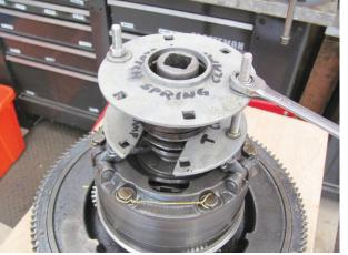
Two scrapped Ford wood wheel hub plates make a handy tool to compress the clutch spring. Notch one to fit into the groove of the clutch shift.
