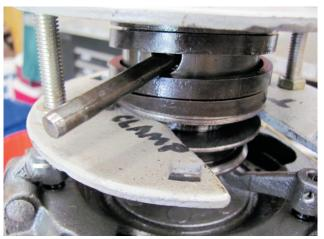
Rotate the spring support to expose the holes and drive the pin out with a drift.
