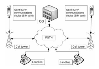
Fig.1 Architecture of Global Service for Mobile communications
