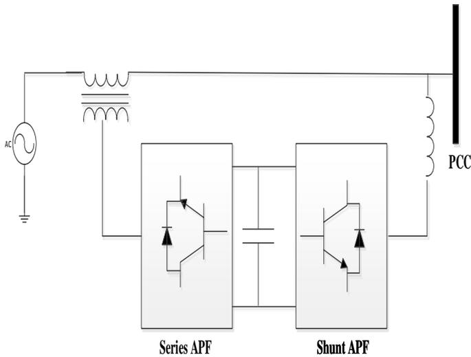
Fig.1: Basic Configuration of UPQC
