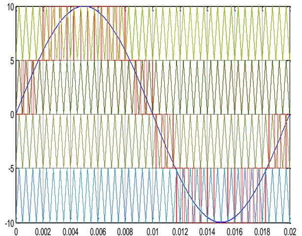
Fig.4: SPWM PD Control Scheme
