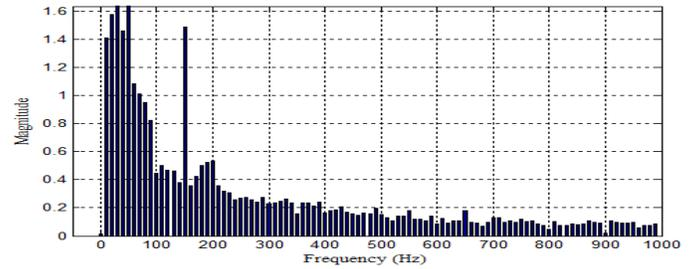
Fig. 14: THD V. Compensation for feeder one
