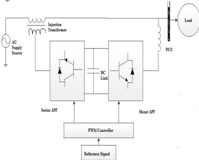
Fig.2: UPQC with controller arrangement
