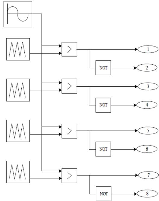
Fig.3: Control scheme algorithm for SPWM
