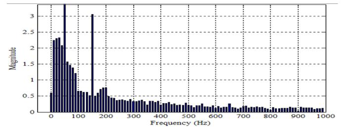
Fig. 16: THD V. injection for feeder one
