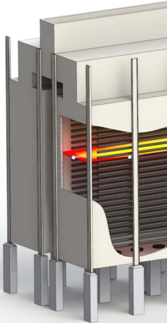
The problem with the image 1 is that most of the heat is concentrated in the center of the heater. The heat needs to be evenly distributed along the entire heater in order to reduce coke build up in the process tubes. Air register adjustments are needed to achieve a more even heat distribution.
