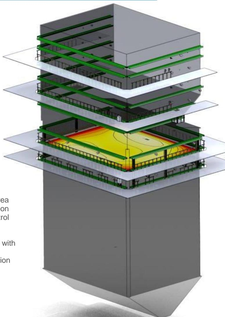
TMS2000 Software show the Isothermal map, Area Map, Trend Graph and Single path. The information on Area Map and Single Map are sent to the Control Room through OPC Output.
