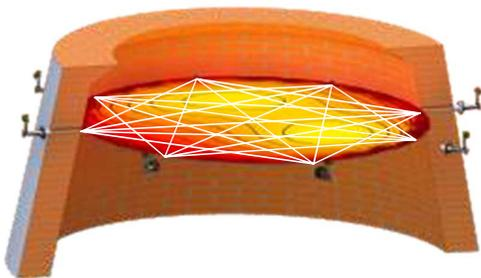
In general, the system consists of 8 identical sender/receiver (transceiver) units, an external control unit and an external evaluation unit. Nitrogen is used for sound generation. With 8 sensors obtain up to 20 paths.
