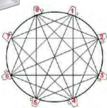
Eight sets of sound wave transmitters and receivers are placed equally spaced around the perimeter of the engine exhaust duct.
