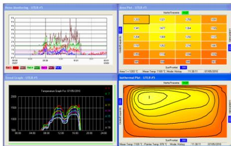
In the boiler startup, the system shown on the screen an isothermal maps, Area Graph Temperature and Noise Graphs Monitoring inside the boiler.
