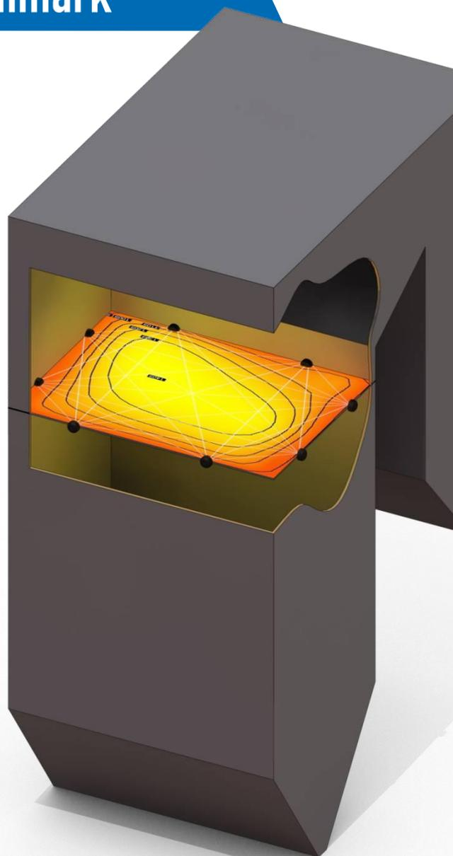
As fouling of the boiler increases and the rate of heat transfer decreases, peak temperatures increase, which increases NOx emissions.
