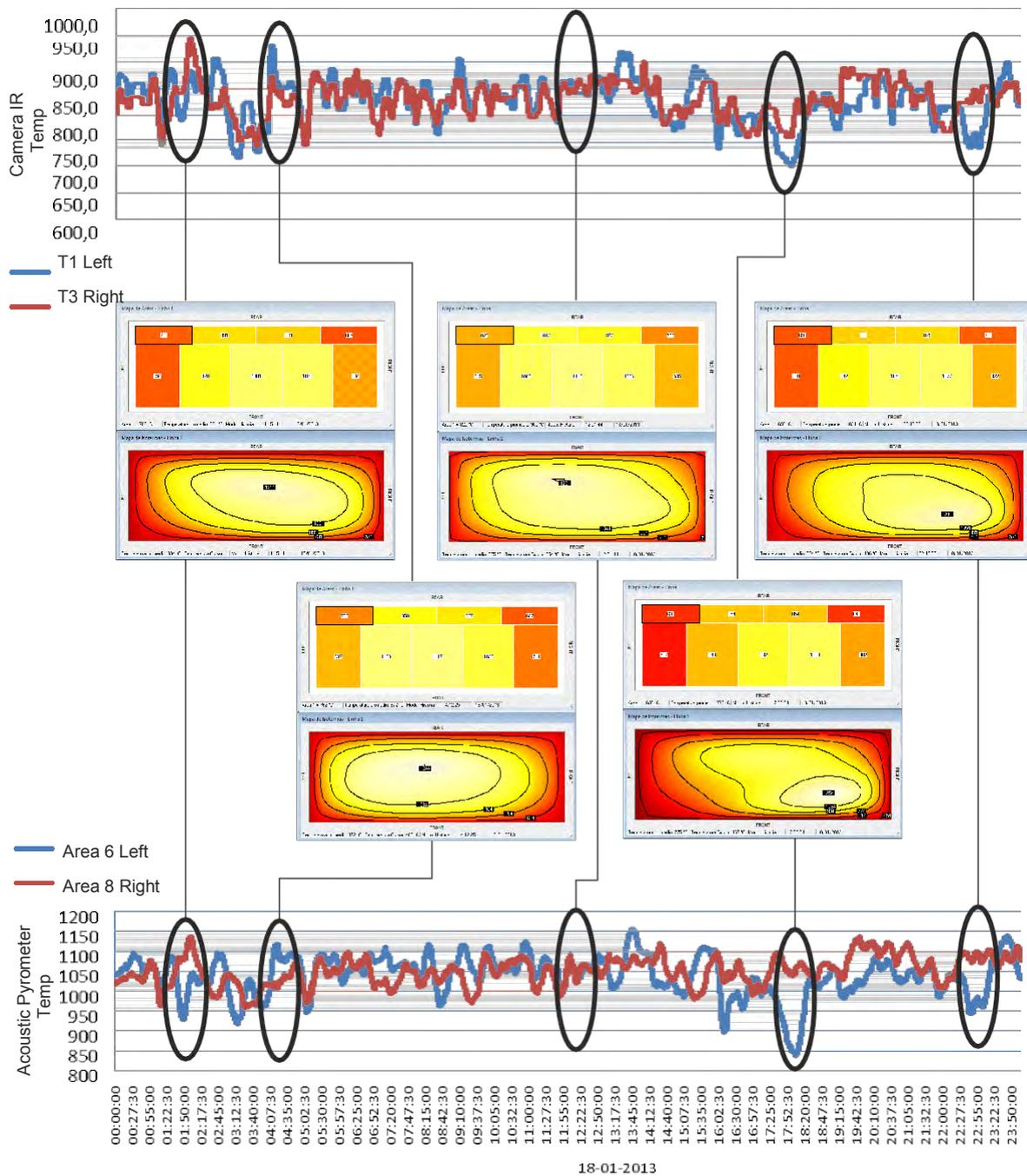
Depending on the fuel type, fuel distribution and air supply, temperature imbalances are typical. The common furnace exit temperatures measured by means of IR Camera and averaged can be used as reference temperatures to a limited extent only as these average temperatures do not say anything about the temperature profile or the imbalances within the injection levels.
