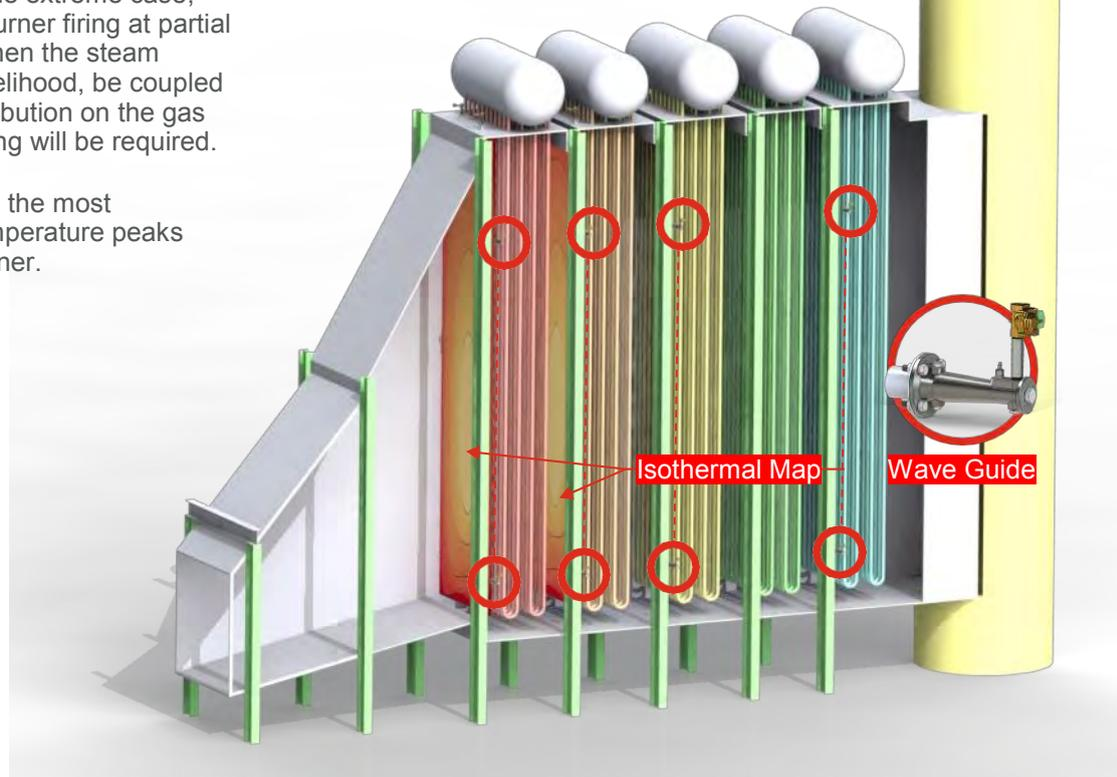
BOILERWATCH® MMP-II-SSX may be installed after the duct burner and before the HRSG. Advantages of this type of installation is the protection of the shock tubes in the HRSG and assurance of correct temperature for the NOx control. Thermal distribution is important for the obtainment of heat transfer in the different regions of the HRSG.
