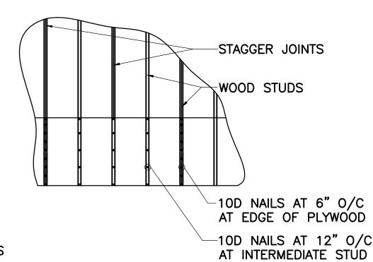
ELEVATION - GABLE NAILING DETAIL AS5.03|2 SCALE : 1/4" = 1'-0"
