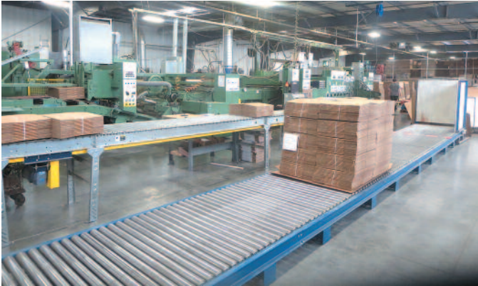
Extensive powered conveyerization by Systec Conveyors has expedited work in process within VPC's plant.
