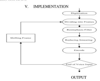
Fig.1: Flowchart - Converting Speech signal into a set parameters suitable for ASR.
