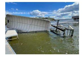
When you put your lift in for the season, do not install the canopy before the boat goes onto the lift. Be sure to coordinate with whoever is installing your lift. Otherwise, this could happen to you, and you would be responsible for damages to the piers as a result.
